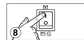
**8. Switch the engine switch to RUN.**
