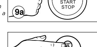
**b. Wireless Remote Start: Hold Start button on wireless remote for 1 second and release.**
