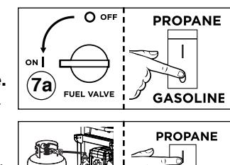
**b. If starting with Propane: Connect propane tank. Push the fuel selector switch to the propane position. Open propane tank valve.**
