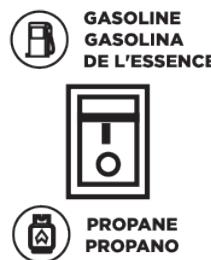
Push the fuel selector switch fully upward for gasoline operation.
