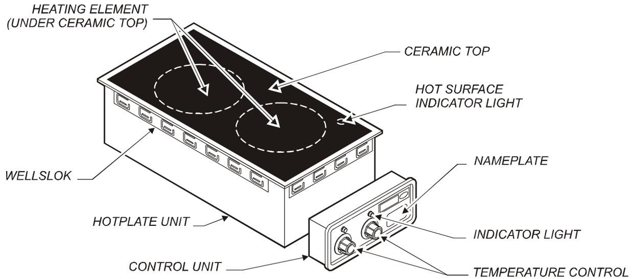
Fig. 1 Built-In Ceramic Hotplate - Features & Operating Controls
