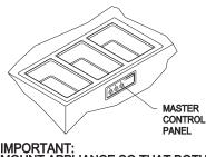
IMPORTANT: MOUNT APPLIANCE SO THAT BOTH THE CONTROL PANEL AND DRAIN MANIFOLD ARE LOCATED TO THE FRONT OF THE FIXTURE.
