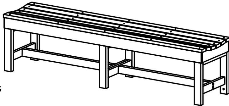
**1)** Attach (1) Support Bar to Leg Support using (2) "A" Bolts as shown
