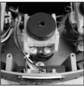
**Step 5:** Remove isolation cap and set aside.
