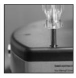
Step 14: Using a Phillips-head screwdriver, fasten screws to top housing cover. Once all set screws have been tightened and top housing cover is secured on top housing, replace screw covers on all screws.
