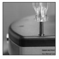
**Step 3:** Using a Phillips-head screwdriver, remove screws from top housing cover.
