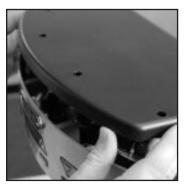
**Step 4:** After all screws and washers have been removed from top housing cover, lift the cover and place at rear of unit.
