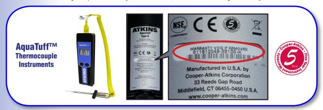
The AquaTuff Thermocouple Instrument above, serial number <u>011612</u>049-35100-K, was manufactured on January 16, 2012.
