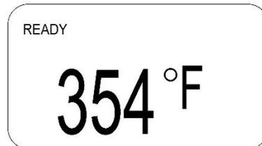
*Although the heating element is programmed to stop at 350° - 354°F, the oil temperature can go as high as 365°F due to the circulation of the oil in the oil pot.*
