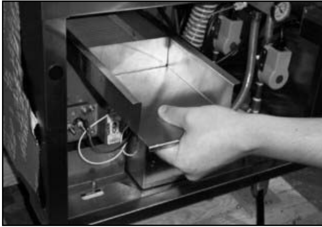
Removing upper (wash) strainer.
