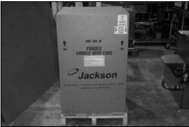
Packaged unit should be visually inspected for damage.
