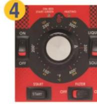
**4** Press FILTER switch to engage the motor/pump. Allow the oil to cycle for a few minutes until the oil and fryer are clean.
