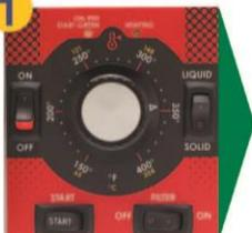
Fill fry tank with oil. Press the power switch **ON**. The red light will come on.
