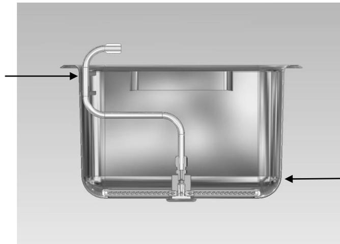
**Filter Screen Lays Flat On Bottom of Filter Pan**
