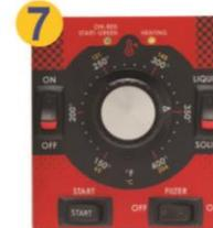
**7** Once the level of the oil has been checked and verified, press the START switch. The red light will turn to green. The burners or heating elements will automatically turn back on and the fryer will resume heating. Yellow light will display when heating.
