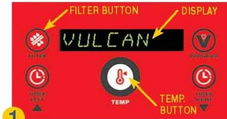
**1** Make sure that the Power Switch is in the "ON" position. Fryer must have power to operate the motor/pump. Fryer Temperature should be between 300-350 Degrees Fahrenheit. RECOMMENDED: ADD OIL TREATMENT MEDIA.
