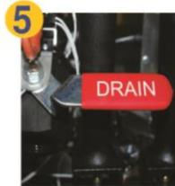
**5** Close the drain valve slowly allowing the oil to fill the fry tank with clean oil. The burners or heating elements will not turn on at this point. Allow the oil to fill back into the fry tank from the filter pan. It is normal to see a few air bubbles during this process.
