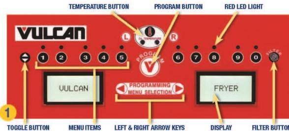
**1** Make sure that the Power Switch is in the "ON" position. Fryer must have power to operate the motor/pump. Fryer Temperature should be between 300-350 Degrees Fahrenheit. **RECOMMENDED: ADD OIL TREATMENT MEDIA.**
