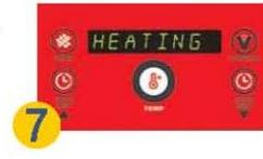
After pressing the TEMP button the fryer resumes heating. **HEATING displays.**
