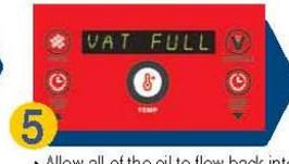
**5** Allow all of the oil to flow back into the fryer from the filter pan. It is normal to see air bubbles in the tank towards the end of filtering. When the filter pan is empty, push the FILTER button to turn off the motor/pump. Oil level should be between the Min/Max lines on the tank back. **VAT FULL displays.** (Display is asking if the tank is full).
