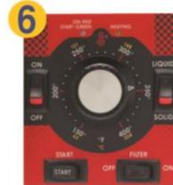
**6** When the filter pan is empty push the FILTER switch to turn off the motor / pump. Oil level should be between the MIN and MAX lines.
