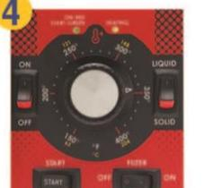
Press the **START** switch and fryer will begin to heat. The burners or heating elements will cycle on and off through the melt cycle. When temperature reaches 135° F the burner or heating element will stay on until set temperature is reached. The red light will change to green. When the fryer calls for heat the yellow light with come on.
