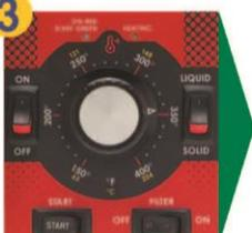
Move the **MELT** switch to the correct shortening being used: Solid or Liquid.
