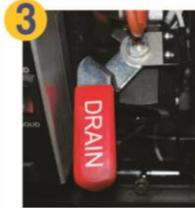
**3** Open the drain valve slowly allowing the oil to drain down into the filter pan. The burners or heating elements will automatically turn off.
