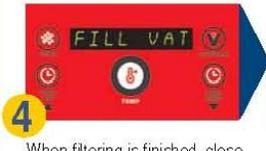
**4** When filtering is finished, close the red drain valve by turning the red drain handle. **FILL VAT displays.**
