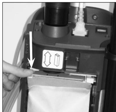
3. Push downwards at the edge to the left of the plastic holder, so that the bag loosens from the vacuum inlet of the machine.
