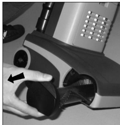
3. Grasp at the bearing block and pull it out from the brush housing.
