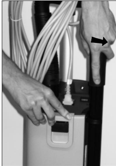
1. Push the machine to upright locked position. The brush will be lifted up from the surface. Then slide the wand out of its holder.
