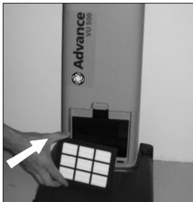
3. Grasp at the filter frame and then insert the new HEPA filter to the cleaner by pushing it in place. (Never touch the filter media of a HEPA-filter! Doing so may cause a loss of performance of the HEPA-filter).
