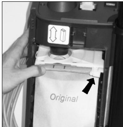
6. Push the bag holder with the new bag upwards, so that the bag inlet fastens to the inlet of the machine. Make sure that the bag is unfolded and will fit in place in the bag housing. Also check that the "no bag" clip is placed to the left so that the lid will be able to close.
