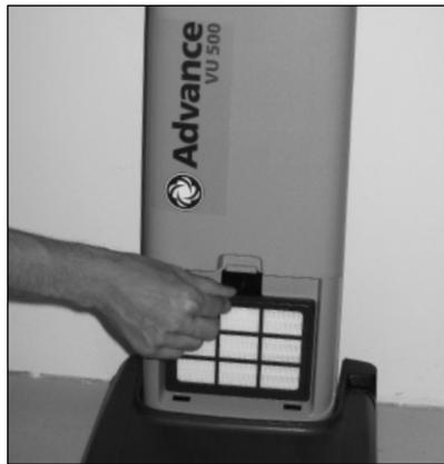
2. Grasp at the filter frame and remove the used and dirty HEPA-filter.
