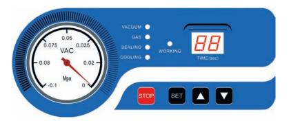
Vacuum Gauge - Indicates the vacuum level inside the chamber.
