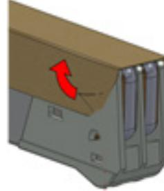
3. Remove the screws on the bottom side of the seal bar.
