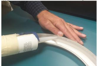
3. Apply a bead of silicone sealant to the inner wall of the ring.
