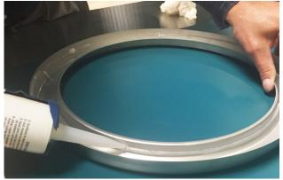
Turn the ring right side up and press it onto the rim of the drop-in until it is firmly seated.
