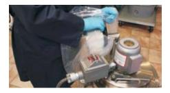
Place a conductive poly liner around the now exposed HEPA/ULPA filter. Carefully remove the HEPA/ULPA filter from the back plate. Gently place the HEPA/ULPA filter into the poly liner. Gently twist the poly liner and then seal it with a tie wrap.
