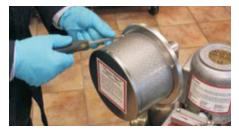
Remove the 3 screws on the HEPA/ULPA housing using a Philips Screw Driver.
