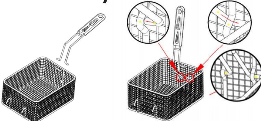
After inserting the end of the handle into place, snap the handle over the top of the basket
