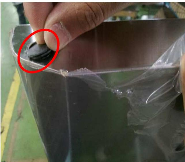
8.Take off unit cover cap from the left-top side of door, then install it in the right side of door hole.
