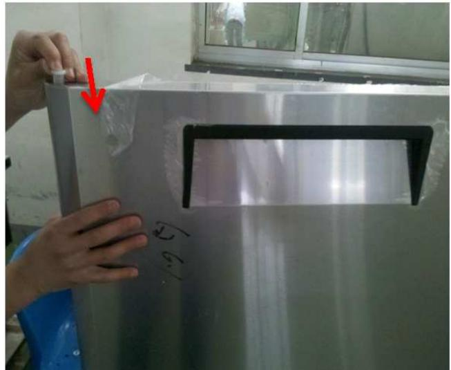
11.Install the door bushing (5mm) in the left bottom side of door
