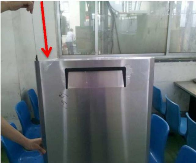
10.Assemble the door bushing (3mm) in the left-top position of door.
