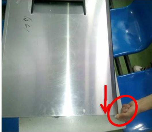
5.Remove door bushing from right-top side of door.
