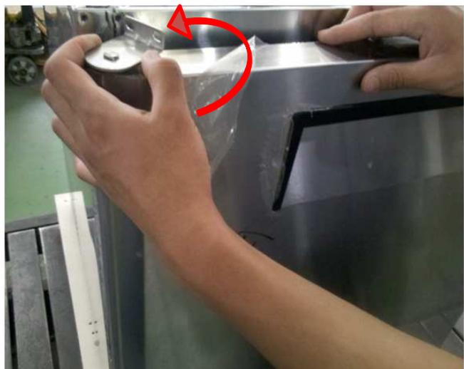
13.Fix the top hinge with screwer
