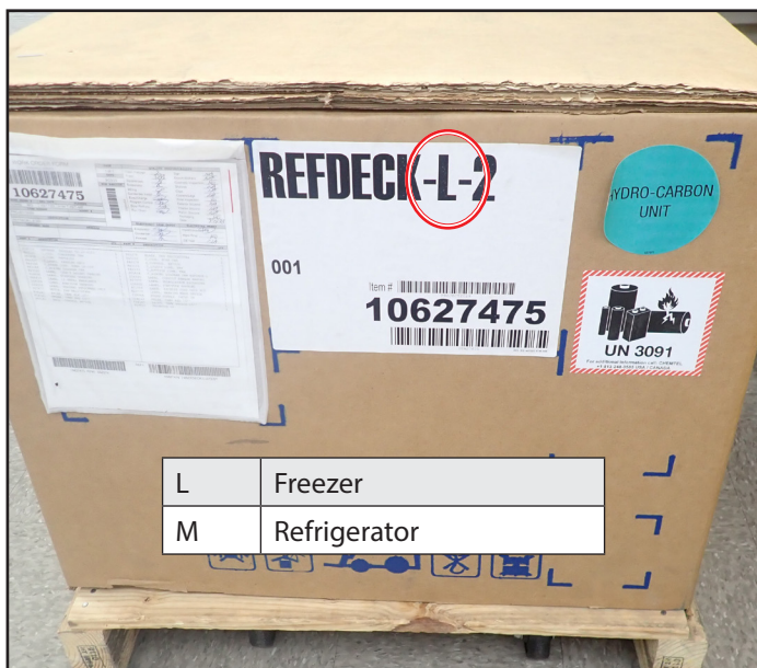
Fig. 1. The letter in the nomenclature identifies the type of refrigeration deck.
