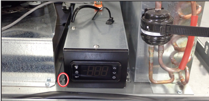
Fig. 1. Temperature control assembly shipping screw screw location.
