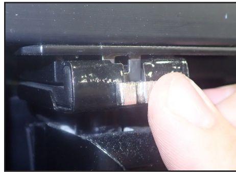
Fig. 21. Insert the hinge retention clip.
