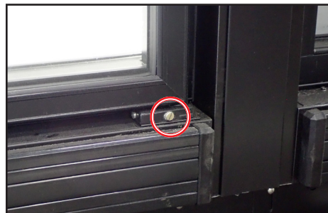
Fig. 24. Door tension adjustment screw location. Clockwise turn: Decrease door tension Counterclockwise turn: Increase door tension
