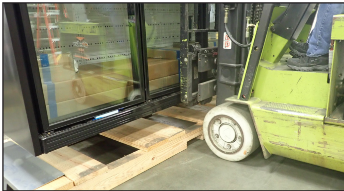
Fig. 6. Lift the unit with a forklift.
