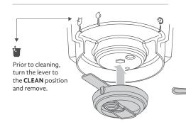
Once it's dry, reassemble on the base of the brewer, as shown, and slide lever to the **BREW** position.
