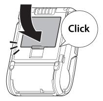
Check the position of the hook to confirm that the battery is securely set. If the battery is not securely set in the printer, it may fall out causing injury or damage to the equipment.
