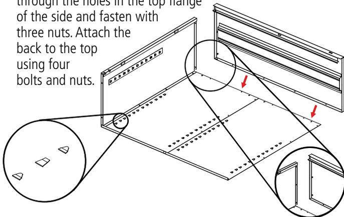
5. Attach the right side (Ref. No. 3) to the back in the same manner as you did in step 3, again making sure that the flange is around the back and that the lances on the shelf adjustment strips are pointed in the same direction as those on the back and left side. Push the side panel up so the studs in the top go through the holes in the top flange of the side and fasten with three nuts.
