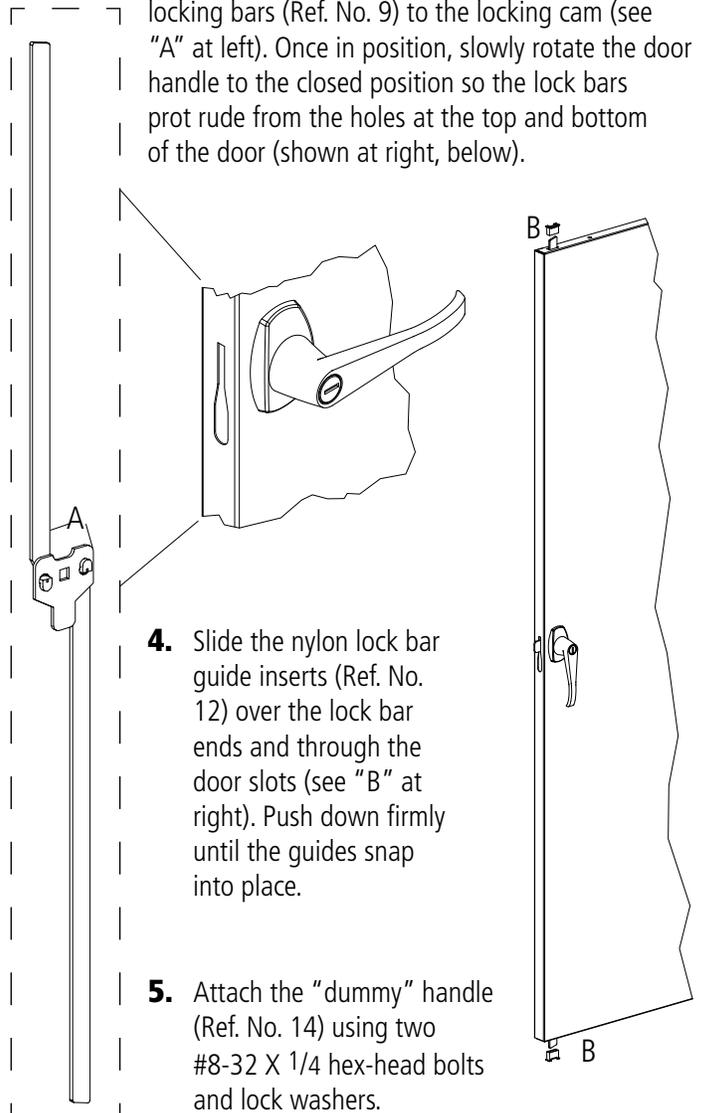
4. Slide the nylon lock bar guide inserts (Ref. No. 12) over the lock bar ends and through the door slots (see "B" at right). Push down firmly until the guides snap into place.
