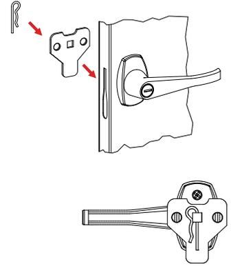
3. With the handle still in the open position, hook the locking bars (Ref. No. 9) to the locking cam (see "A" at left). Once in position, slowly rotate the door handle to the closed position so the lock bars protrude from the holes at the top and bottom of the door (shown at right, below).
