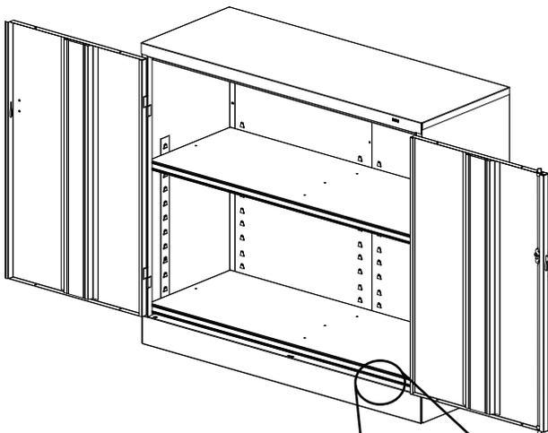
10. Cabinet must be level for doors to open and close properly. Insert a flathead screwdriver into the two leveling holes and turn the screws until the cabinet is level. The cabinet is now ready for use.
