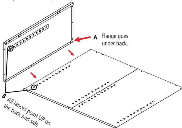
4. Attach the top (Ref. No. 8) to the unit by sliding the outer flange over the back of the unit and the side flange to the side panel on the unit. The threaded studs should go through the holes in the top flange of the side and fasten with three nuts. Attach the back to the top using four bolts and nuts.
