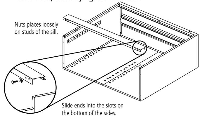
7. Place the rear flange of the bottom shelf (Ref. No. 5) into the bottom lances of the back. The flange with two holes should face the front, hanging over the sill.
