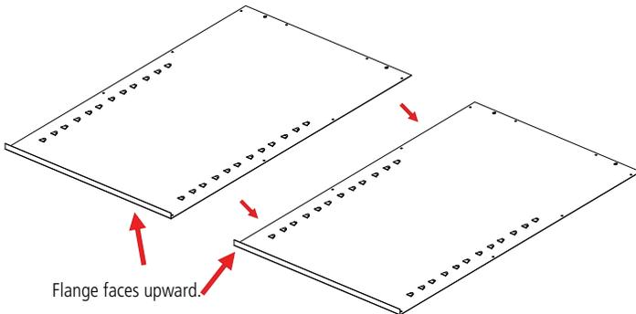
3. Attach the left side (Ref. No. 2) to the back by placing flange (A) around the back and bolting tightly together with four bolts and nuts. Be sure that the lances on all the shelf adjustment strips (B) point in the same direction.
