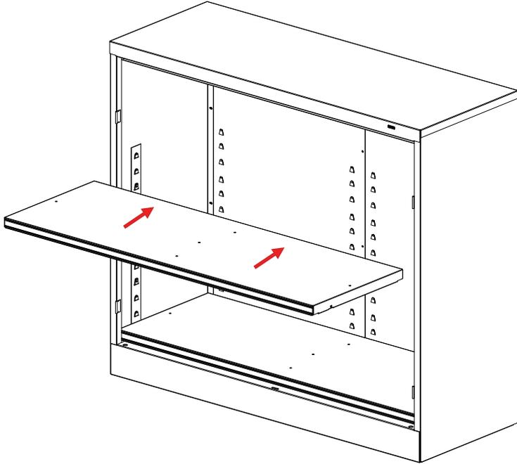
**NOTE:** In order to place the shelf, you must first tilt the shelf slightly to the left or right before inserting into the unit.
