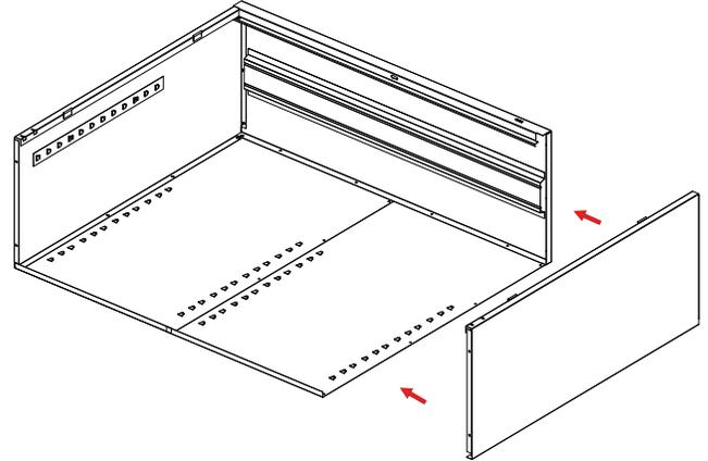
6. Attach the sill (Ref. No. 4) to the sides. Place a nut (Ref. No. 19) loosely on each of the studs and slide the ends of the sill into the slots on both sides of the unit. Then, securely tighten the nuts.
