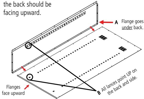
Attach the left side (Ref. No. 2) to the back by placing flange (A) around the back and bolting together with seven bolts and nuts (Ref. Nos. 19 & 20). Be sure that the lances on all shelf adjustment strips (B) point in the same direction.
