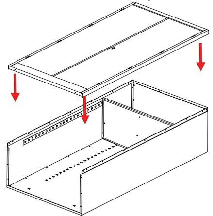
7. With the door and frame assembly in place, attach it securely to the unit by opening each door, one at a time, and securing the frame assembly using two bolts and twenty nuts. This will require attaching nuts to the nine pre-welded studs along each side, plus two bolts and nuts along the top.
