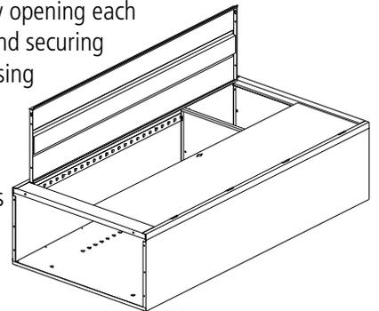
8. Place the the bottom (Ref. No. 7) in the lowest notch of the shelf adjusting strips on the back. Make sure the flange with two holes faces the front, and that it is over the flange of the frame sill. If necessary, you may push out on the side walls to enable the bottom to more easily slide into position. Attach the shelf securely by bolting the bottom to the frame sill with two bolts and nuts.
