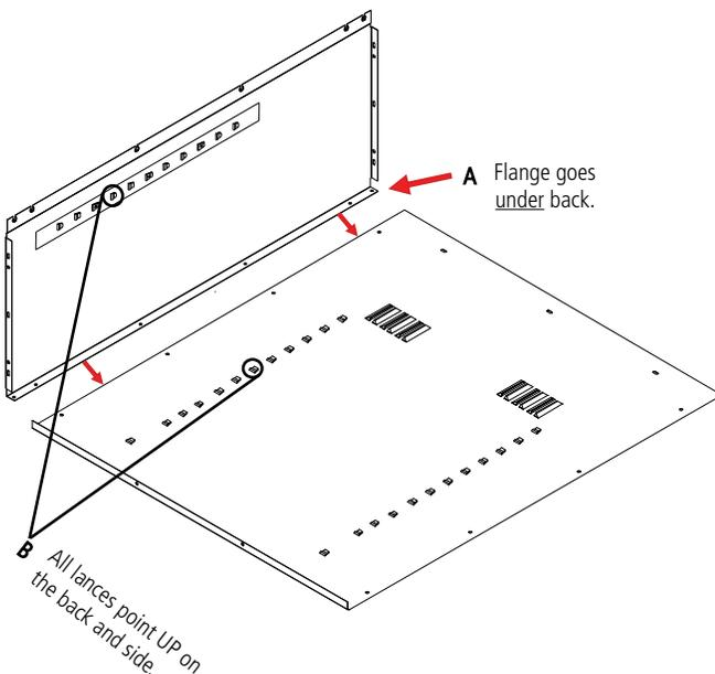
4. Attach the right side (Ref. No. 3) to the back in the same manner as in step 3, again making sure that the flange is around the back and that the lances on the shelf adjustment strips are pointed in the same direction as those on the back and left side.
