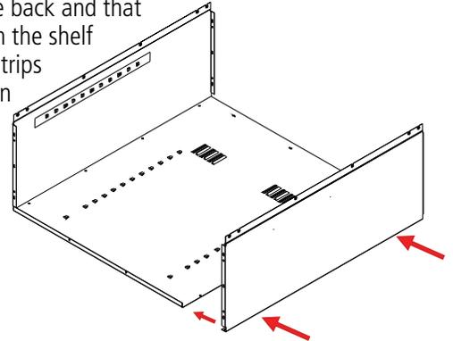
5. Insert one shelf (Ref. No. 4) into the approximate center of the unit, inserting the shelf edges into the lances on all four shelf adjustment strips. Be sure that the channeled edge of the shelf is toward the cabinet front.
