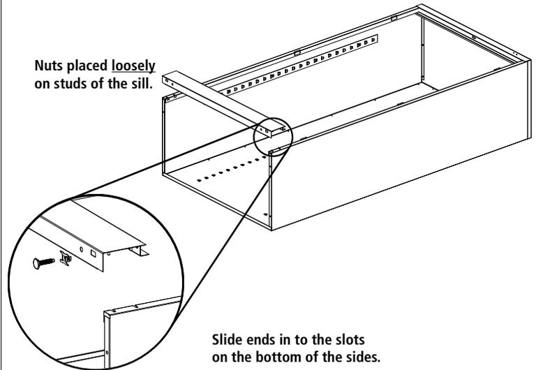
7. Place the rear flange of the bottom (Ref. No. 7) into the bottom lances of the back. The flange with two holes should face the front, hanging over the sill. Insert the bolts through the bottom and still with the head facing the front of the unit. Secure with two nuts.
