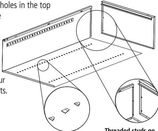
Threaded studs go through the holes in the flange at the top of the side.
