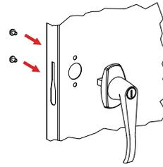
1. Place the locking handle (Ref. No. 11) on the right hand door and fasten with two #8-32 X 1/4 hex-head bolts and lock washers, provided with the handle.
