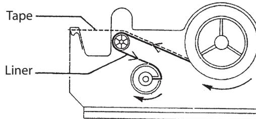
If the spool (1) doesn't rewind the liner promptly, it is necessary to increase the friction torque, turning the knurled knob (2) clockwise, until the liner is completely rewound.
