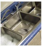
STEP 7 Transfer these parts to a three compartment sink for cleaning. Fill the first sink with a soap solution using a mild detergent, the second sink is used for clean rinse, and the third sink with a sanitizer solution (75°F warm chlorine solution of 50-100 ppm).
