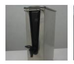
STEP 1 Once a week, fill the dispenser with a chlorine solution (75°F warm chlorine solution of 50-100 ppm).
