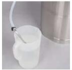
If using bottled concentrate, place the draw tube in the container with soap solution.
