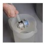
Sanitizing the BIB 14. connector, tubing metering valve:
