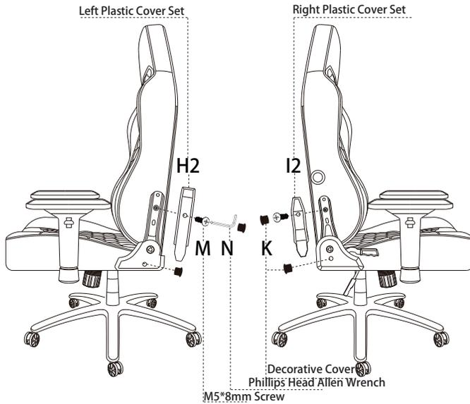
Attach the Left Plastic Trim Cover (Part H2) and Right Plastic Trim Cover (Part I2) using (2) M5\*8mm Screws (Part M). Tighten using Phillips Head Allen Wrench (Part N). Insert (4) Decorative Covers (Part K).
