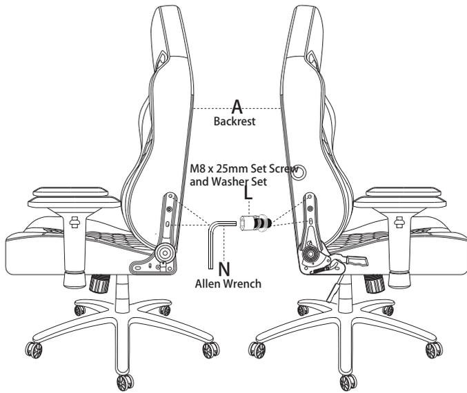
Attach the Backrest (Part A) to the Seat using (4) Set Screw and Washer Sets (Part L) These are preinstalled in the back. Tighten with Allen Wrench (Part N).
