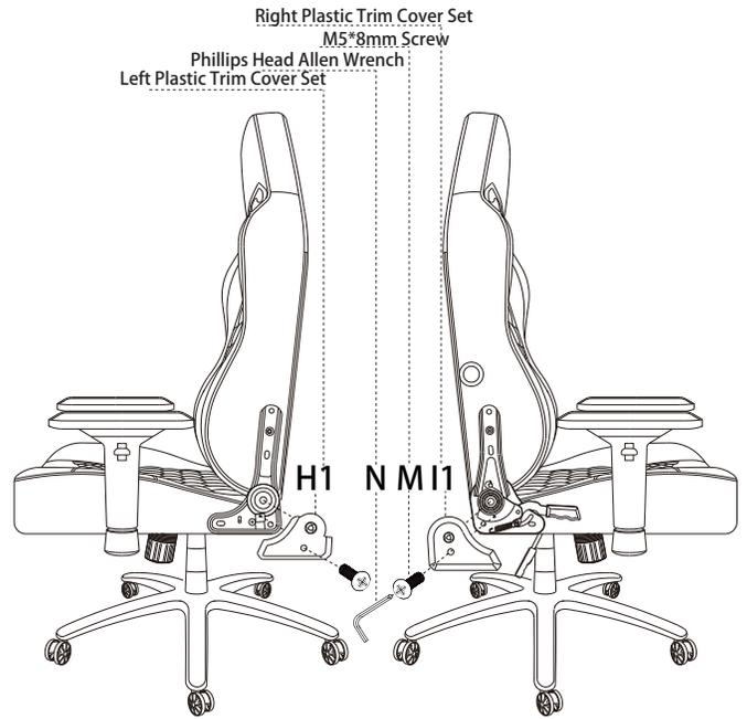
Attach the Left Plastic Trim Cover (Part H1) and Right Plastic Trim Cover (Part I1) using (2) M5\*8mm Screws (Part M). Tighten using Phillips Head Allen Wrench (Part N)
