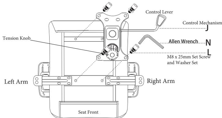
Remove (4) Set Screw and Washer Sets (Part L) from the underside of the Seat (Part B) and align the holes of the Control Mechanism (Part J) with the holes in the seat ensuring control lever is facing the Right Arm and Tension Knob faces the Seat Front. Tighten with Allen Wrench (Part N).
