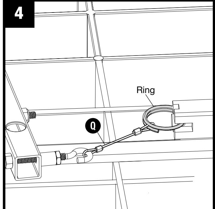
Thread lanyard (Q) onto Hooks connected to (P).
