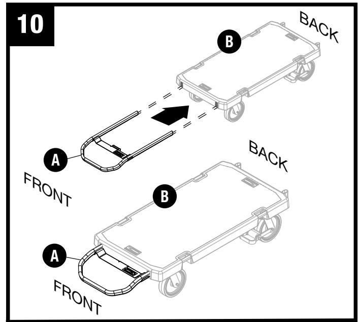
Insert handle (A) into slots on back of the unit. Push down and snap into place.
