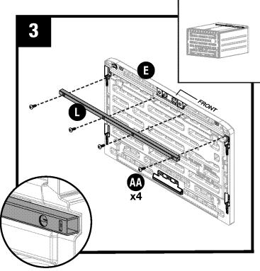
Attach support tube (L) to top panel (E) using four screws (AA). Large hole of support tube must face out.
