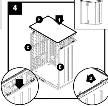
Align slots on top panel (E) with tabs on side panel (C/B). Lower top panel and lock in place by sliding panel towards front. Top will overhang front slightly.
