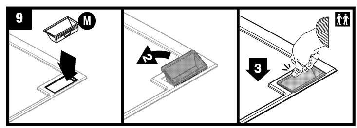
Place door on a flat hard surface. Lower (M) into left door. Insert on an angle. Hole for lock must be facing inside of cabinet. Push down hard on center of handle to snap in place. Repeat with right door.
