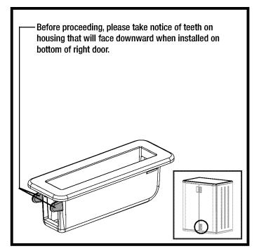
Insert door latch housing (K) into bottom right door (G) and snap into place. Insert door latch (J) into door latch housing. Push latch pin down so it is fully seated in latch housing. Push down with force until you hear a snap. Slide latch up and down to confirm it slides properly.
