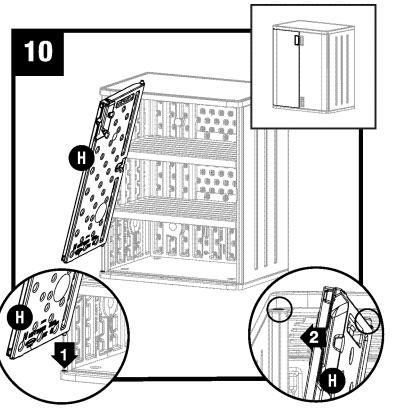
With left door (H) in the open position, place door into hinge receptacle on bottom left of cabinet. Insert hinge pin under top panel and slide to the left into hinge receptacle. Repeat with right door (G).
