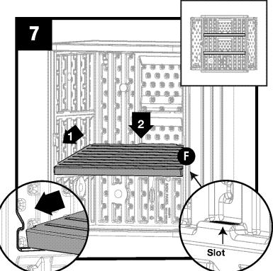
Tab on shelf must engage with slot on inside panel for each shelf. Push side panels inward to engage.
