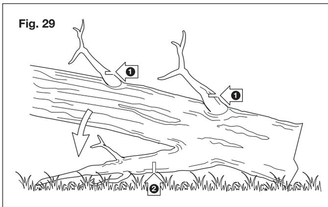
**⚠️ WARNING!** Pay special attention to where the branches are lying on the ground and recognize the following risks: 1). the branches may be under tension; 2). the direction in which the branch will fall may differ from that anticipated; 3). the tree may be unstable after the branch has been cut.
