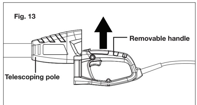
**⚠ WARNING!** Always make sure that both the cutting head lock and the handle lock are locked securely before using the pole chain saw.
