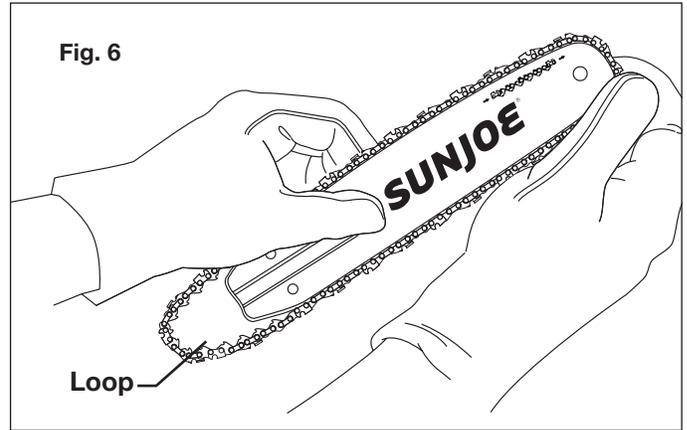
6. Hold the chain in position on the bar and place the loop around the sprocket. Fit the bar flush against the mounting surface so that the bar studs are in the long slot of the bar and the adjusting pin is in the chain tension pin hole (Fig. 7).
