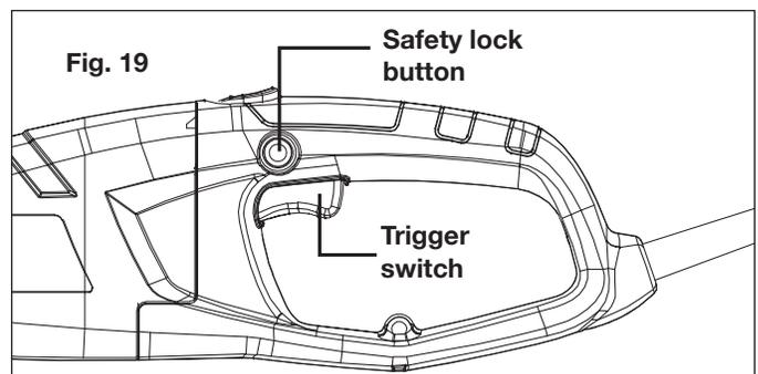
5. To turn the tool OFF, release the trigger switch (Fig. 16).
