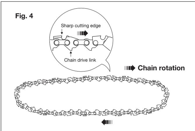
5. Starting at the tip, mount the chain drive links into the bar groove, leaving a loop at the back of the bar. The chain will loosely fit until it is placed on the sprocket (Figs. 5 & 6).
