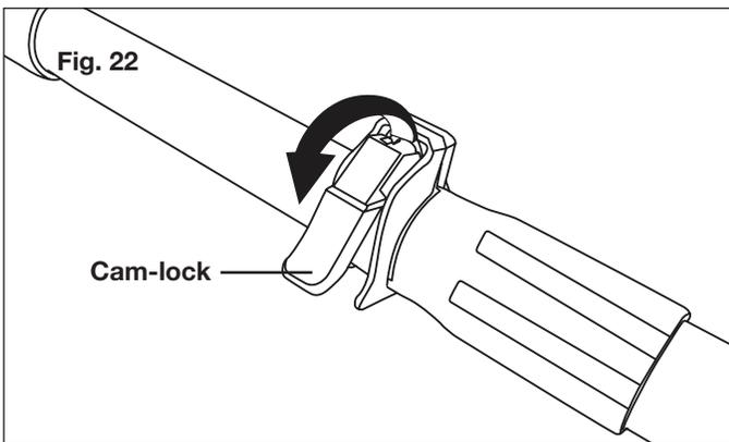
**⚠ WARNING!** Failure to lock the telescoping pole cam-lock as directed could result in personal injury.
