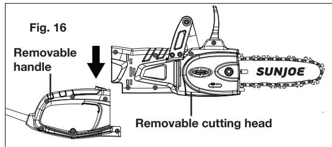
**⚠ WARNING!** Always make sure that the handle lock is locked securely before using the chain saw.
