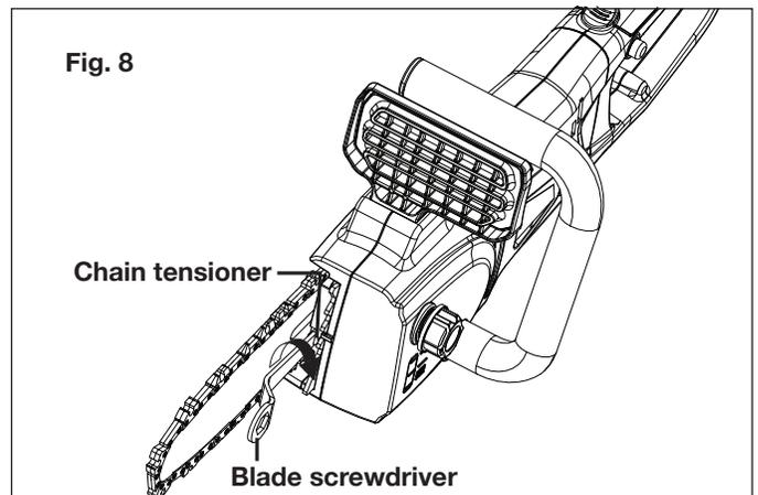
8. Replace the chain/sprocket end cover. Tighten the end cover nut, but leave the bar free to move for tension adjustment.
