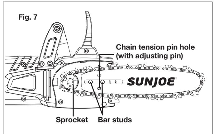
7. Adjust the chain tension as needed by adjusting the chain tensioner screw with the supplied flat-tip blade screwdriver. Make sure to align the chain tensioner screw with the pin hole (Fig. 8).
