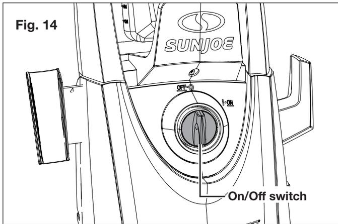
14. Check that the electrical supply voltage and frequency (Volt/Hz) correspond to those specified on the pressure washer rating plate. If the power supply is correct, you may now plug the pressure washer into the power outlet (Fig. 15).
