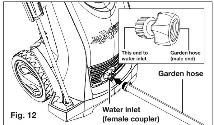
**⚠ WARNING!** The machine is not suitable for connection to the potable water main.
