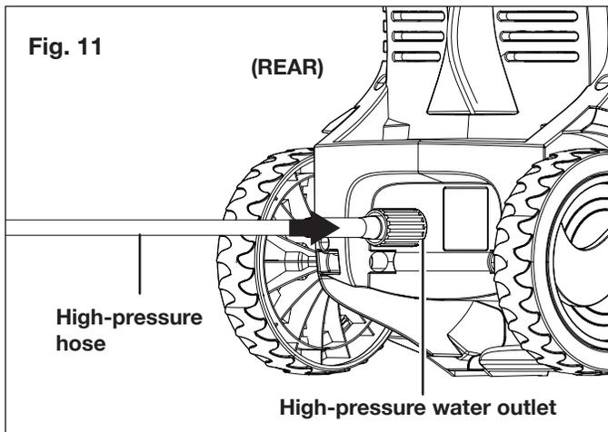
**⚠ WARNING!** Keep hose away from sharp objects. Bursting hoses may cause injury. Examine hoses regularly and replace if damaged. Do not attempt to mend a damaged hose.
