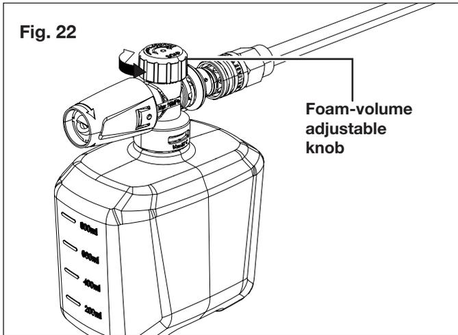
5. Apply detergent from the bottom to the top of the dry surface to be cleaned. Applying detergent in this manner will dissolve dirt most effectively.
