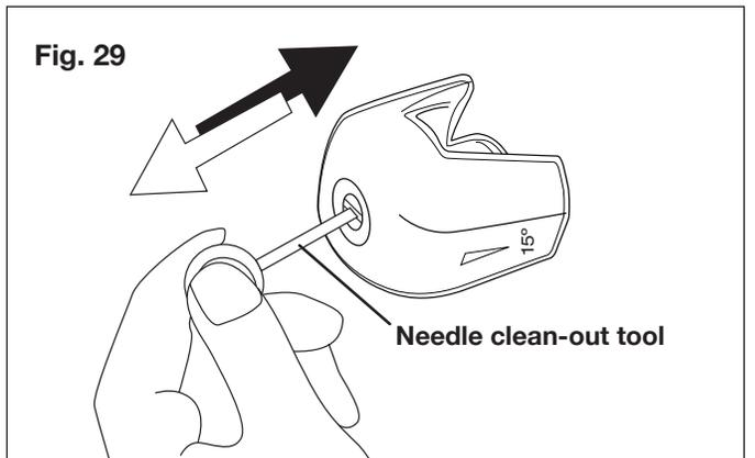
3. Remove additional debris by back flushing water through the nozzle and stainless steel lance. To do this, place the end of your garden hose (with water running) to the tip of the nozzle, pushing water and debris out of the back opening of the nozzle and stainless steel lance.
