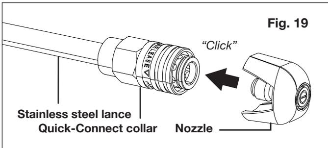
To disconnect a nozzle from the stainless steel lance once the cleaning job is complete:
