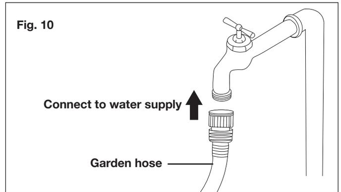
**⚠ WARNING!** Do not connect to potable water system.
