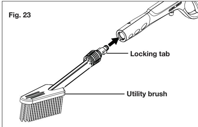
3. Once aligned, push the utility brush into the trigger gun, twist counterclockwise to lock into place.
