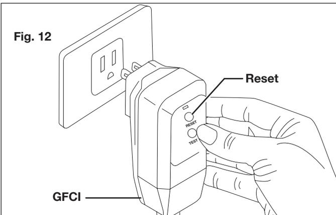
**NOTE:** The GFCI may need to be reset when first plugged into the electric outlet. Press the "Reset" button until the power light indicator on the GFCI illuminates when plugged in.
