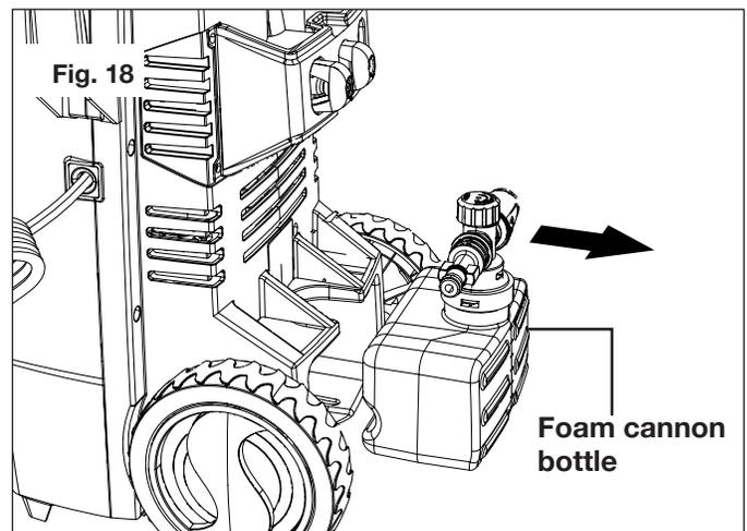
2. Remove the cap. Fill the bottle or mix as recommended by detergent instructions (Fig. 19), and secure the cap back into place. Replace it back on the unit.
