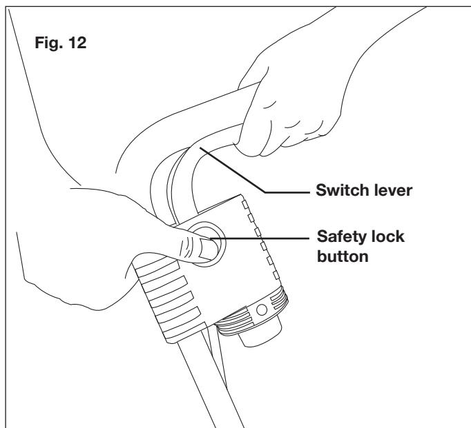
4. Once the machine powers on, release the safety lock button and proceed with operation, gently lowering the mower down into the cutting position (Fig. 13).
