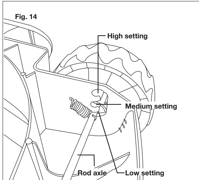
4. The wheel axles can be placed into 3 different cutting heights: low (will cut grass the shortest), medium, and high (Fig. 14).
