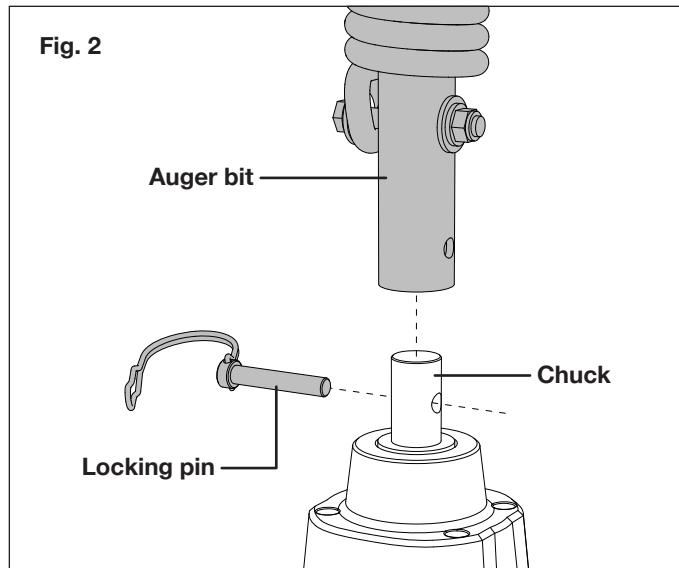
3. Flip the wire latch over the locking pin to secure it in place (Fig. 3).
