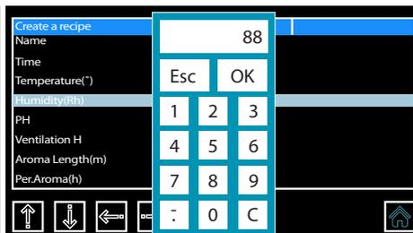
12. For the majority of the parameters, you will be working with the keypad to modify its value.
