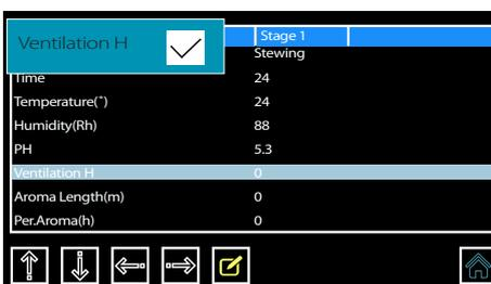
14. By pressing on the empty box you will place a check mark inside, setting the fan on high-speed for this stage when needed.
