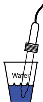
3. With the pH 4 field highlighted in yellow, Place the pH probe into the cup with the 4.01 solution, be sure to hold the probe so that it does not touch the bottom/sides of the cup. The correct pH 4 value will sit in the 1300 -1500 range. Once the value has stabilized press the pH 4 button to save and continue.
