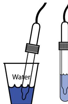
5. With the pH 7 field highlighted in yellow, Place the pH probe into the cup with the 7.01 solution, be sure to hold the probe so that it does not touch the bottom/sides of the cup. The correct pH 7 value will sit in the 1900 -2300 range. Once the value has stabilized press the pH 7 button to save.
