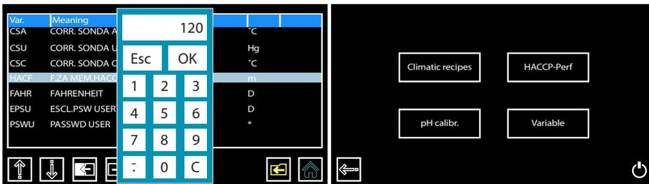
4. Use the keypad to enter the new value. The range of values that can be set are between 1.....240 minutes (m). Once value is set press OK. Press the folder/left facing arrow icon to save and exit the variables page.
