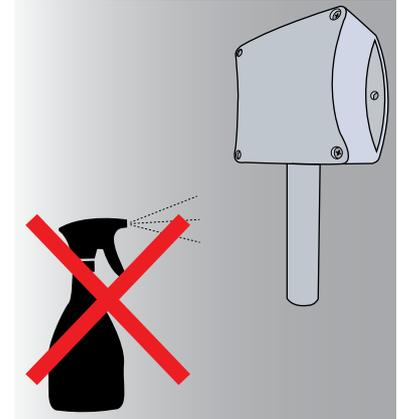
Before beginning, be sure to remove all food product and Stagionello® accessories, such as guides, grills/shelves, and hanging rods. Using a mild detergent, spray all internal surfaces including vent holes, corners, steam output valve, door/s and glass panel/s. **Never spray Humidity probe directly.**
