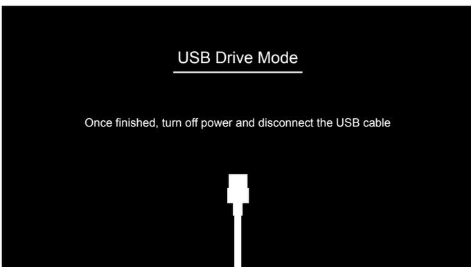
Once the 2 devices have been connected, power up your Stagionello®. Your controller will now display the communication mode screen, and a new window will open on your computer. Copy/Cut the firmware file from its current location and paste into newly opened window. A small uploading window will appear and will take several seconds (depending on computer) to begin. Once completed, power down your Stagionello and disconnect the micro USB cable from the controller.
