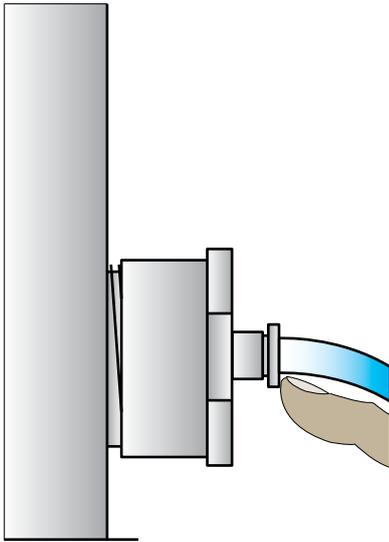
1. Push on ring around water tube and pull hose.
