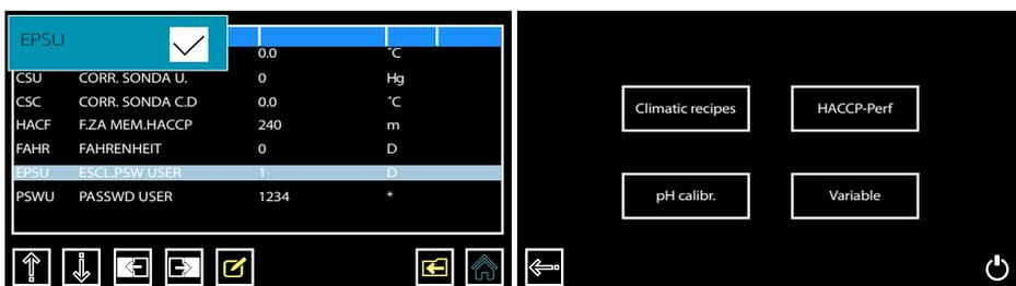
4. By pressing on the empty box you will place a check mark inside, activating the screen lock. Press the folder/left facing arrow icon to save and exit the variables page.
