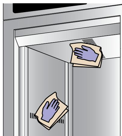
Using paper towel, wipe down all internal surfaces that may have residual moisture. Thoroughly drying your Stagionello® will ensure its proper functionality and hygienic state.
