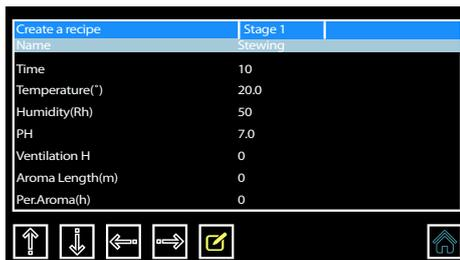
10. Use the down arrow to scroll through the recipe parameters, one by one, and adjust according to your needs.
