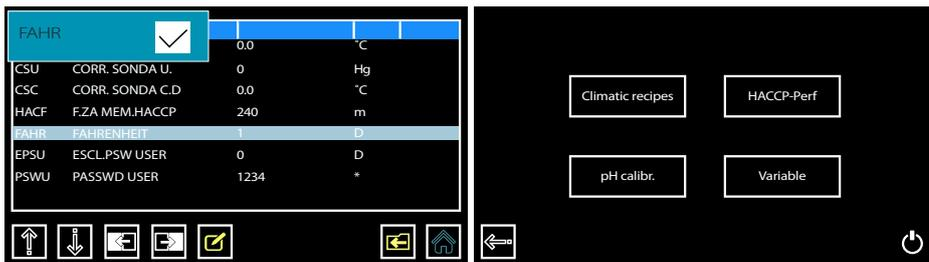
4. By pressing on the empty box you will place a check mark inside, locking in Farenheit as the new unit of measurement. Press the folder/left facing arrow icon to save and exit the variables page.
