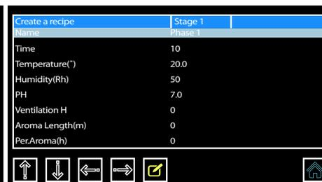
8. On this page you have \*16 fields that can be modified (\*with the exception of Free Variable this should be left 0). With the name field highlighted in red, press the pencil icon to activate the keyboard and set the name for this stage.
