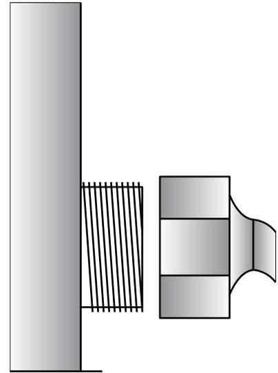
3. Connect using a standard water hose connection 3/4", do not over tighten
