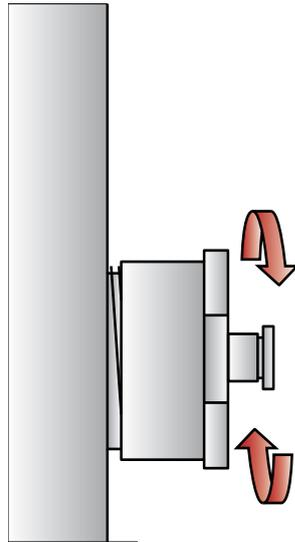
2. Unscrew and remove reducer.
