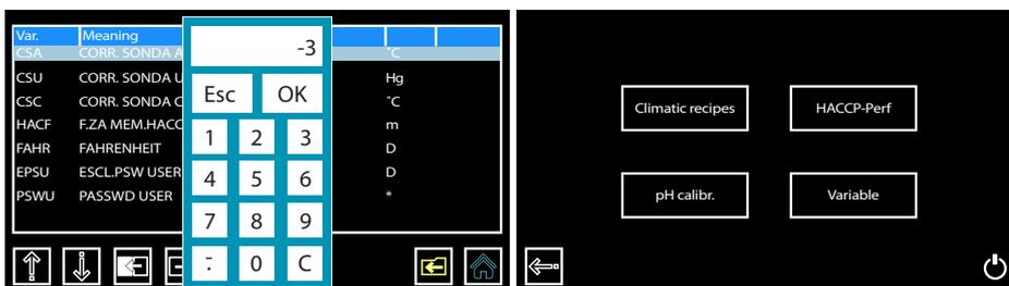
4. Use the keypad to enter the new value. The range of values that can be set are between -20...0...+20. Once value is set press OK. Press the folder / left facing arrow icon to save and exit the variables page.
