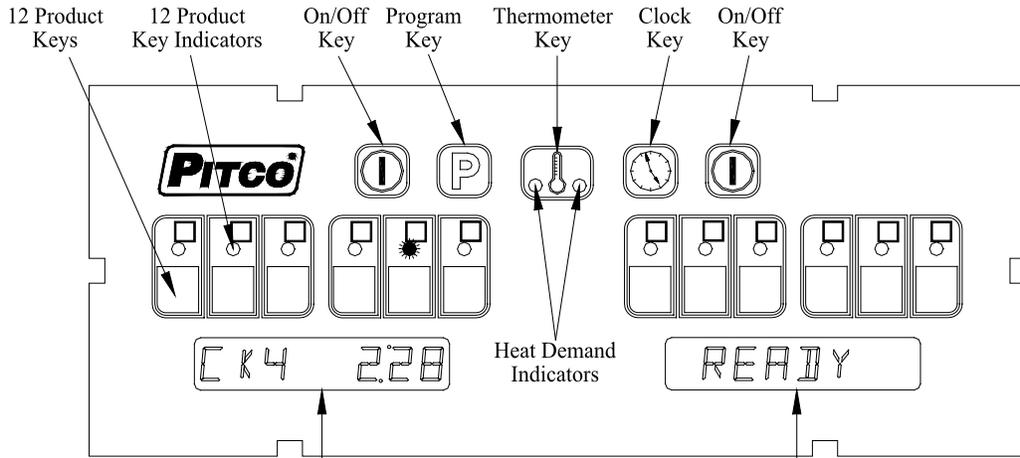
Displays show current operation. Throughout this text, a left only display will be printed as [CK4 2:28]. When both left and right displays should be interpreted together, this text will show them as [CK4 2:28] [READY ].
