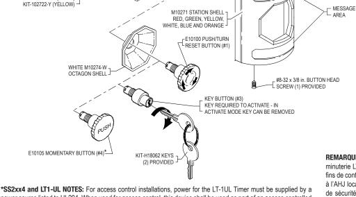
power source listed to UL294. When used for access control, this device shall be used as part of an access controlled egress door system. It is up to the local AHJ to allow use of this device in place of an automatic sensor. For higher security installations, lower time limits should be used. For SS2xx4 and LT1-UL the enclosed timer is to be used and installed per the enclosed LT-1UL installation sheet. \*SS2xx4 and LT1-UL maximum rating 30 VDC 3A.
