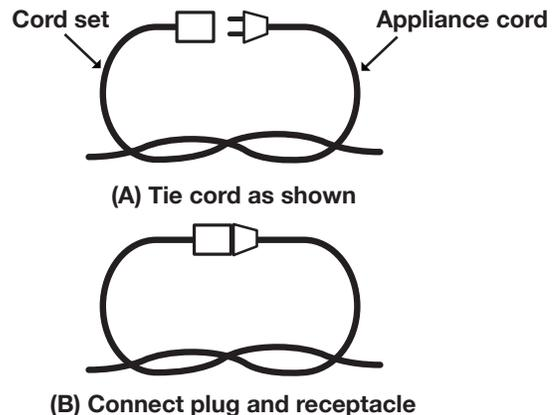
7. Do not abuse the cord. Never pull the pressure washer by the cord or yank the cord to disconnect it from the receptacle. Keep the cord away from heat, oil, and sharp edges.
