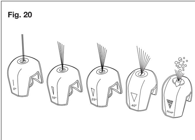
I) The 0° intense-jet nozzle (red) is an extremely powerful nozzle that delivers a high-pressure, pencil-point jet stream. It is used to cut heavy dirt deposits in a small, concentrated area. It is ideal for dissolving stubborn substances, like tar and grease spots on concrete, or for removing caked mud from equipment. Use this nozzle to clean hard-to-reach areas including the facades of 2-story buildings or the undersides of lawn mowers and tractors.
