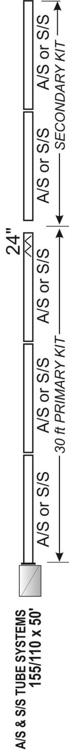
NOTE: FOR FOLLOWING MODELS THE TUBE WITH TURBULATOR(S) IS PACKAGED IN THE 30 FT PRIMARY TUBE KIT, BUT INSTALLS AT VENT END OF SYSTEM
