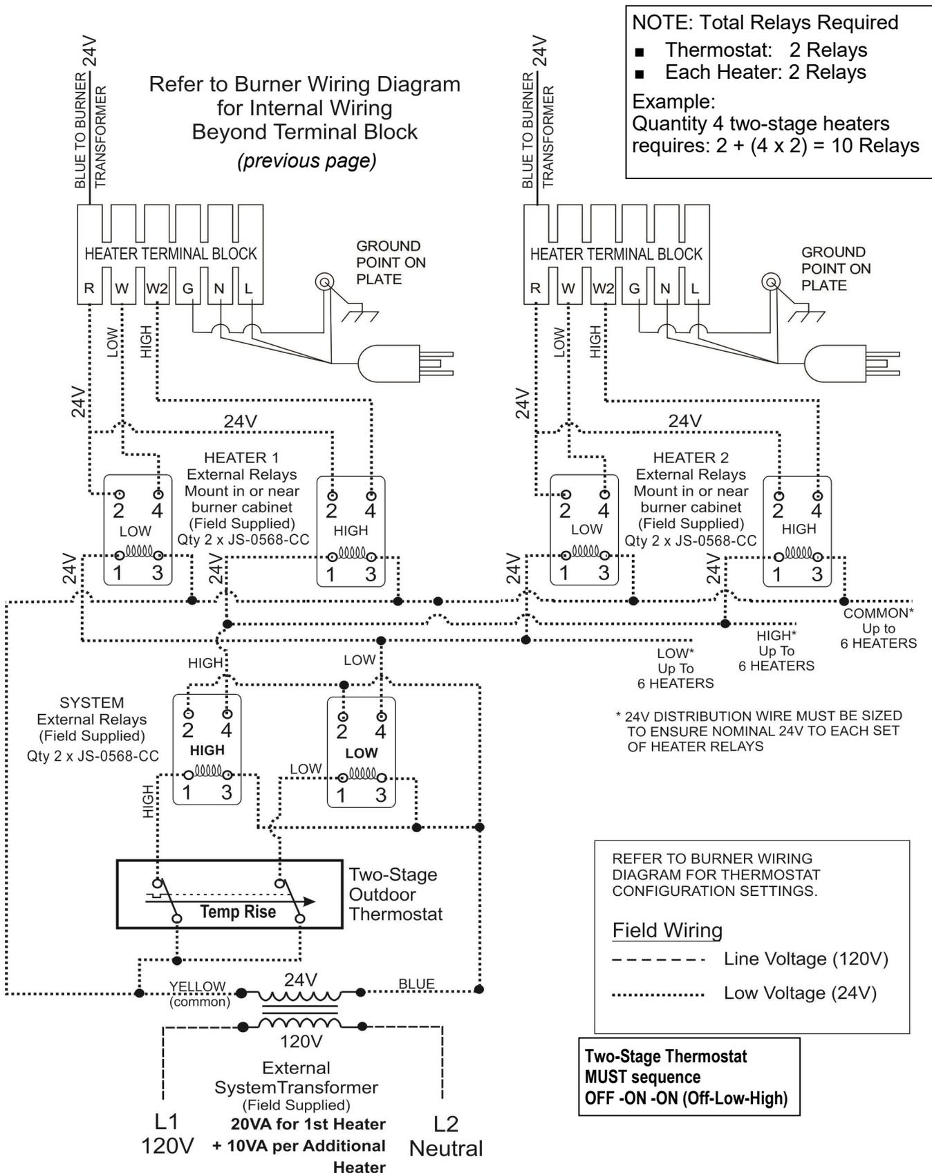
**19. WIRING DIAGRAM: 24V 2-STAGE MANUAL SWITCH CONTROL
