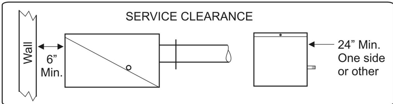
**TABLE 2: GUIDELINES FOR HEATER PLACEMENT: INDOOR SPACE HEATING**
