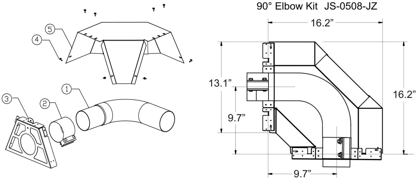
Angle mounting of the reflector system either side of an elbow requires adapter JS-0504-JZ. The elbow always remains in a horizontal orientation.
