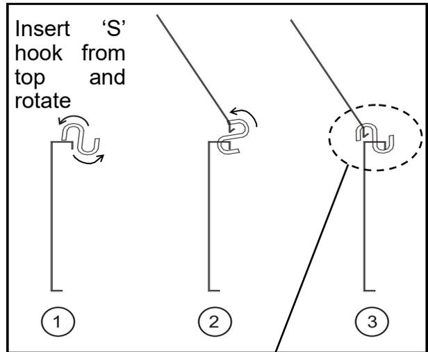
1. Reflector extensions may be installed on one side or both sides of the reflector
