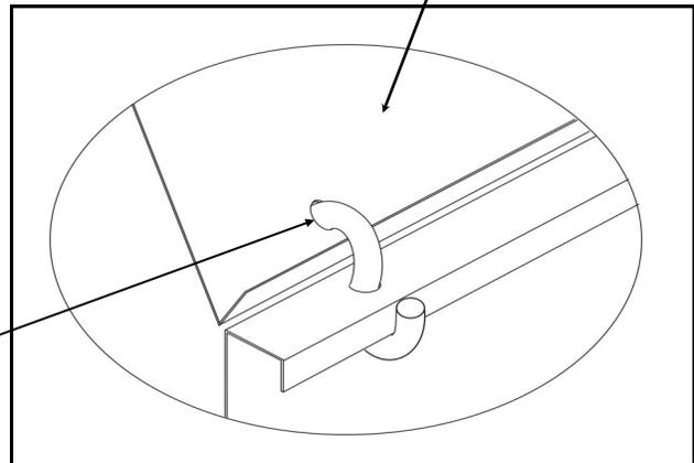
5. Insert "S" hook down through hole in the top of the reflector extension
