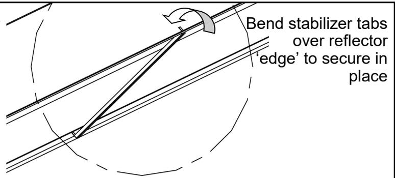
Bend stabilizer tabs over reflector 'edge' to secure in place
