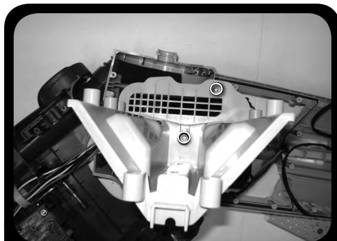
10. Remove air separator - Remove two (2) (M4 x 20mm length) screws
