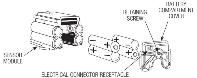
Install Battery Compartment Cover and secure with Retaining Screw. Make certain that Battery Compartment Cover is fully compressed against Gasket to provide a seal; **Do Not** overtighten. Plug the Electrical Connector into the Battery Compartment Cover. Reinstall the Sensor Module onto the Plate. Reinstall the complete Cover Assembly onto the Plate. Tighten the two (2) Screws on top of the unit.
