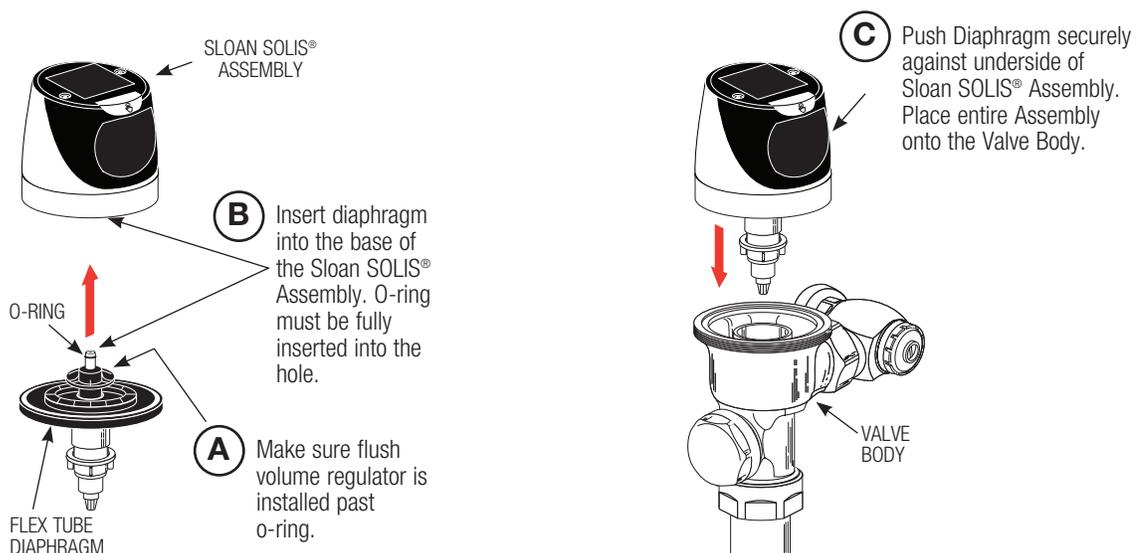
**To facilitate installation, wet the diaphragm assembly (on top or completely).**
