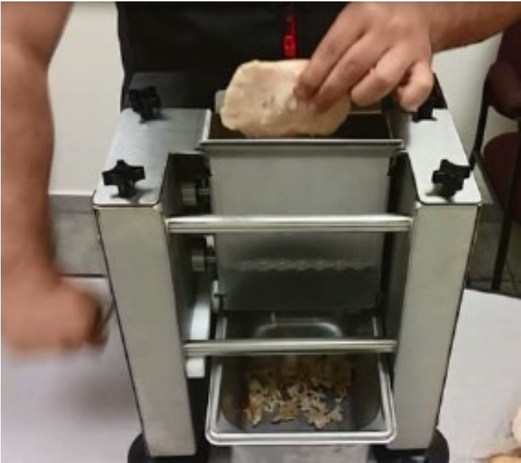
No more than 2 pieces of chicken in shredder at one time. Chicken MUST be cold for the Shredder to work properly.
