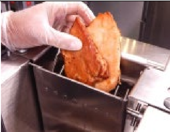
No more than 2 pieces of chicken in shredder at one time. Chicken MUST be cold for the Shredder to work properly.
