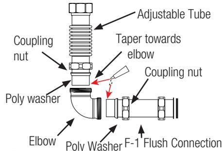
Loctite must cure for 24 hours before turning on water otherwise the Loctite will wash out and joint will leak
