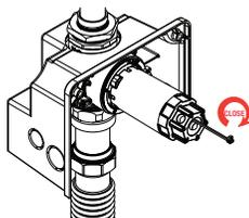
**K** Using adjustment tool, turn activation assembly counter clockwise to open flow of water through the valve.
