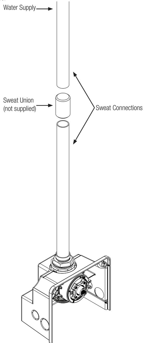
**NOTE: PROPERLY BRACE SUPPLY PIPE AFTER SWEATING CONNECTIONS TO PREVENT VALVE MOVEMENT DURING INSTALLATION AND USE SLOAN RECOMMENDS BRACING VALVE WITHIN 6" OF INLET CONNECTION.**
