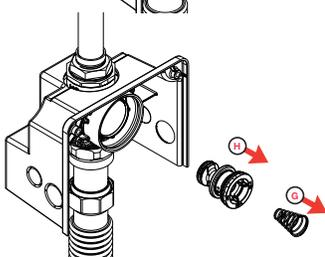
**I** Reinstall activation assembly and press until fully seated. Remove screws.
