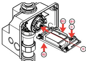
**L** Once lines are flushed clear, turn activation assembly clockwise to shut off water.
