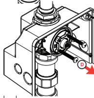
**O** Reinstall piston. Insert smaller sized end first until fully seated.
