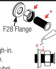
Loctite must cure for 24 hours before turning on water; otherwise the Loctite will wash out and joint will leak.
