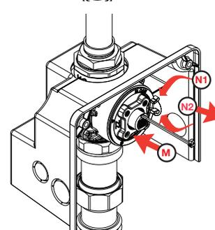
**F** Attached provided 1/4-20 screws to activation assembly. Pull to remove assembly
