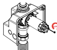
**C** Disconnect Solenoid from Sensor assembly. Pull on end connector to prevent damage to wires.
