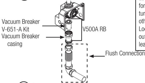
Loctite must cure for 24 hours before turning on water otherwise the Loctite will wash out and joint will leak
