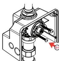
**J** Reinstall Collar. Collar will spin freely in valve body when properly installed.
