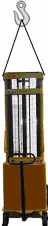
Lifting belt specification— Use polyester lifting sling or nylon sling and hoist with a minimum of 2,000 lb. capacity.
