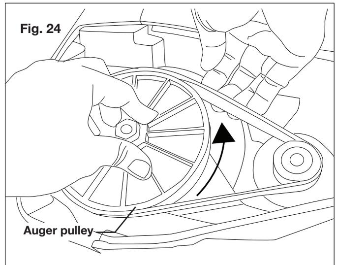
3. Put the belt on the drive pulley first and then place the belt at the lower end of the auger pulley (Fig. 25).
