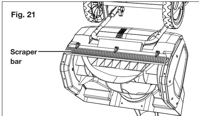
2. Remove the 3 screws that secure the scraper bar to the snow thrower (Fig. 22). Remove the old scraper bar.
