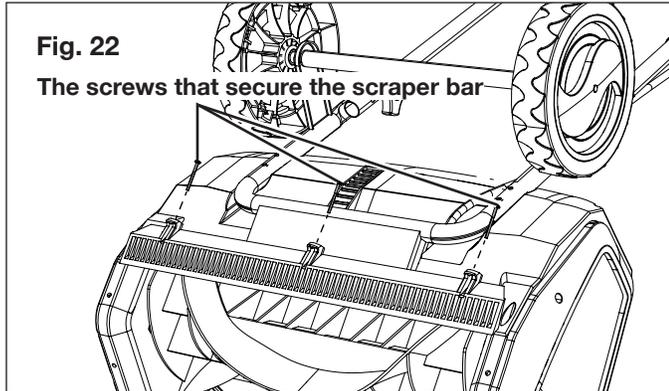
3. Install the new scraper bar and fasten it securely to the snow thrower with the 3 screws.
