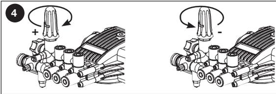
**NOTICE:** DO NOT overtighten the pressure control knob, if overtightened the knob COULD break and result in immediate loss of water pressure and costly repairs to the unit.
