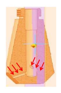
Holes' tilted angles increase milk vortex speed, mixing milk and air in the jug, giving a consistant temperature.
