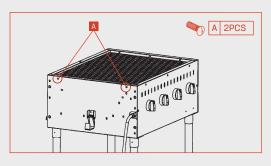
Install Screw-A (2PCS) into the holes in the top of the grill body section.
