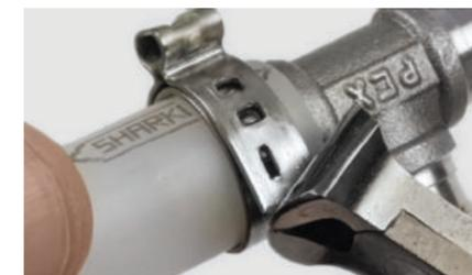
**Note:** The previously clamped section of SharkBite PEX pipe should be cut off before making a new connection.
