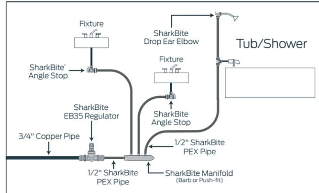
This system uses traditional PEX components (manifolds, barbed fittings, clamp rings, etc.) and offers the total lowest material cost. When you need special configuration fittings, such as drop ear elbows, SharkBite push-fittings offer greater speed and efficiency than traditional barbed fittings while costing about the same.
