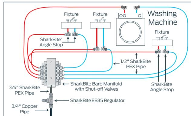
This system uses a central manifold to distribute water to fixture and appliances. One dedicated plumbing line is run to each fixture/appliance for both hot and cold supply lines.
