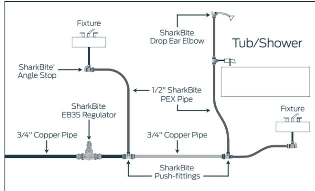
This system uses SharkBite PEX pipe and push-fittings. It offers the absolute fastest and easiest way to get from meter to fixtures.
